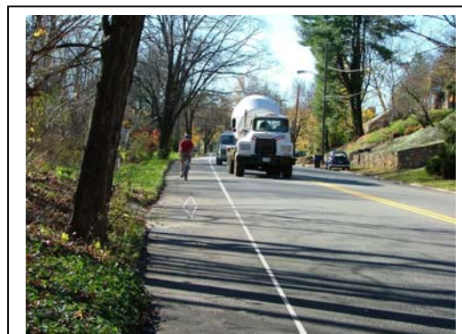
Figure 6.3 Using the BCI and basic graphics software, a bike lane was inserted into the travel lane for “visioning” purposes.
