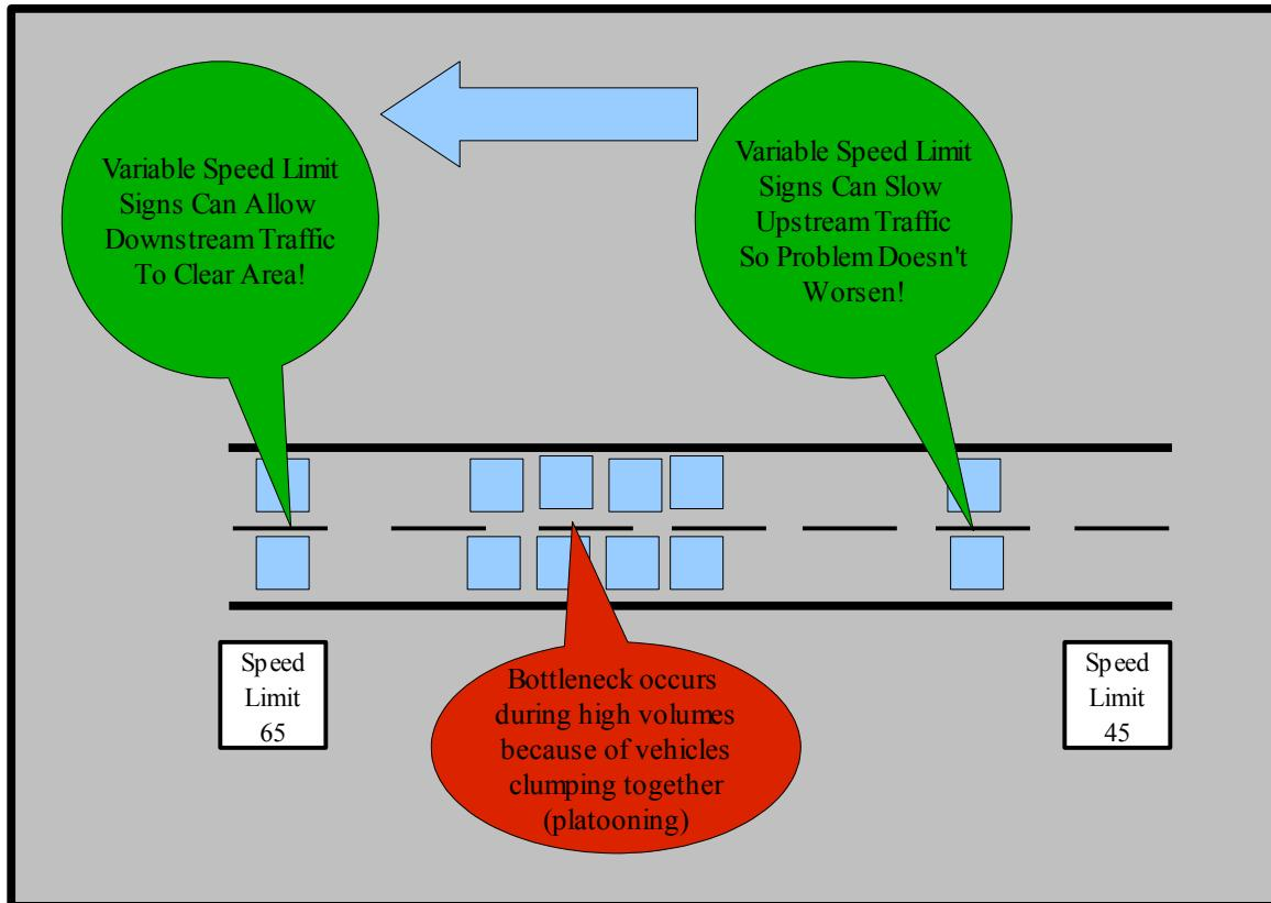
A variable speed limit zone on an interstate or divided highway section would allow speed limit adjustments in response to traffic flow conditions. Images on the following pages have been edited to include elements of a traffic flow management system. The basic relationship between “before” (unaltered) and “after” (altered) images is presented below.
