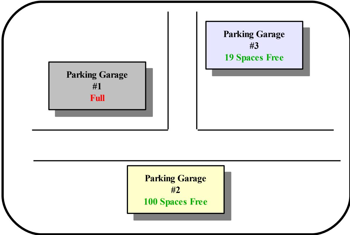
In this concept Variable Message Signs would warn drivers which parking garages are full and direct drivers to parking garages with available space. This system could be combined with a common parking pass or common parking payment system to facilitate parking management. The basic relationship between “before” (unaltered) and “after” (altered) images is presented below.
