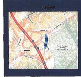
Signal at off ramp will eliminate weave.
