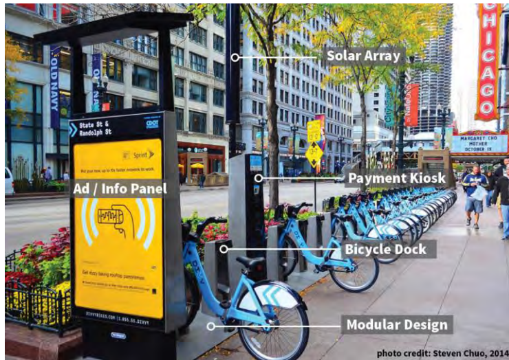
Figure 7.5.1-1 | Typical Dock Based Stations
