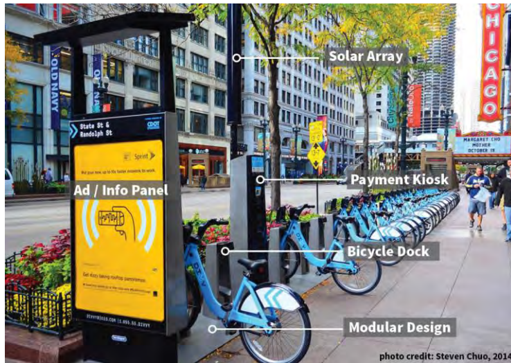
Figure 7.5.1-1 | Typical Dock Based Stations
