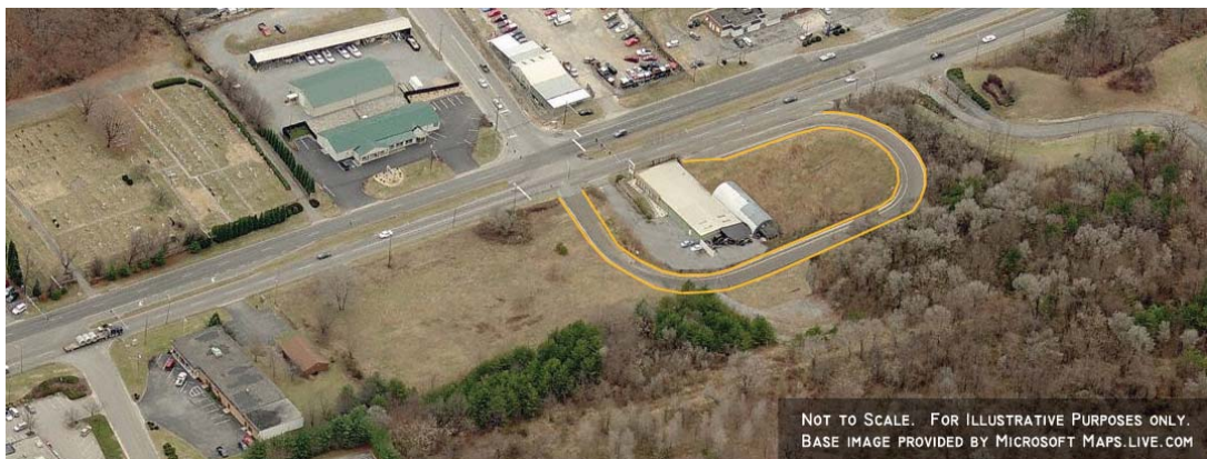
Computer illustration of right hand access lanes (i.e. "jug handle") to accommodate left hand turns - highlighted in yellow
