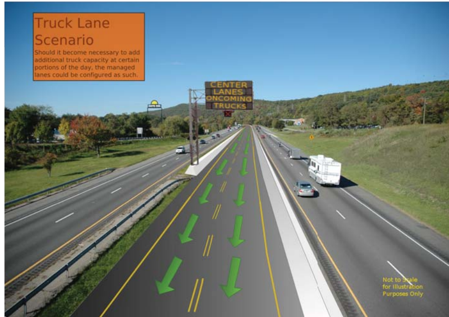
Photo-Simulation of managed lanes in current I-81 median configured for peak truck demand. Managed lanes could be coupled with a Variable Message Sign (center).
