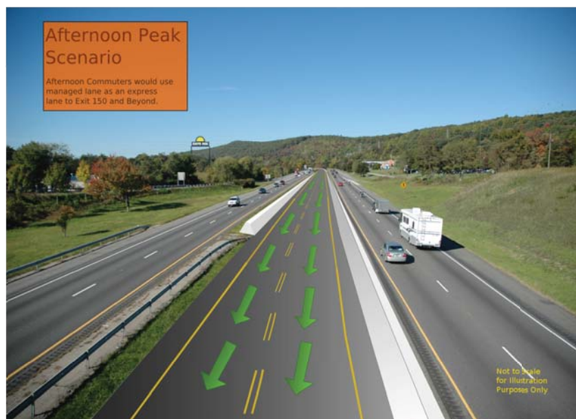
Photo-Simulation of managed lanes in current I-81 median configured for afternoon peak commute out of Roanoke Metropolitan Area.
