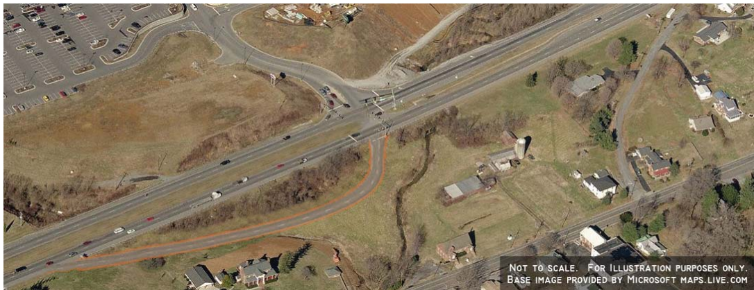
Computer illustration of right hand access lanes (i.e. "jug handle") to accommodate left hand turns - highlighted in orange
