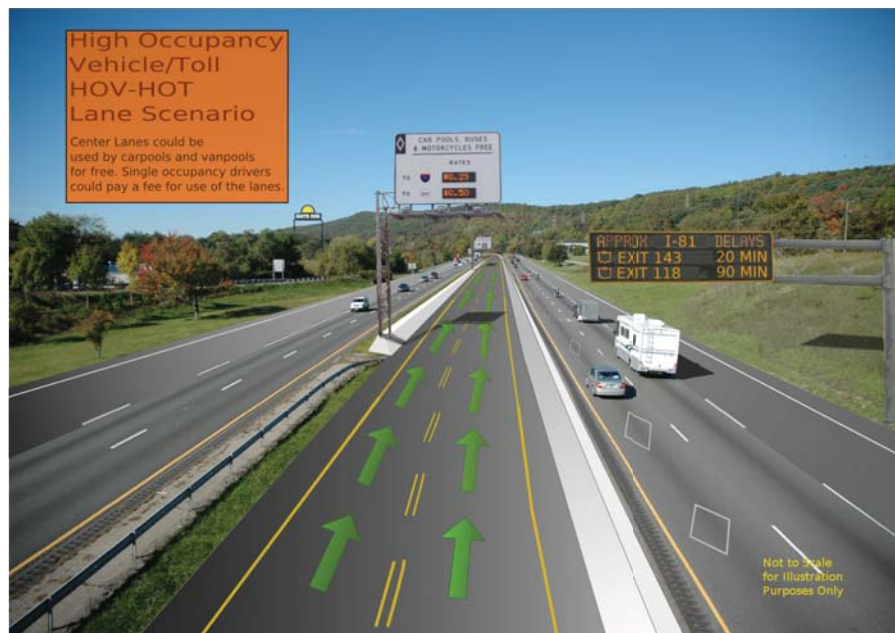
Photo-Simulation of managed lanes in current I-81 median configured for morning High Occupancy Toll (HOT) peak commute. Managed lanes could be coupled with a Variable Message Sign (center), and additional High Occupancy Vehicle (HOV) outside lanes.
