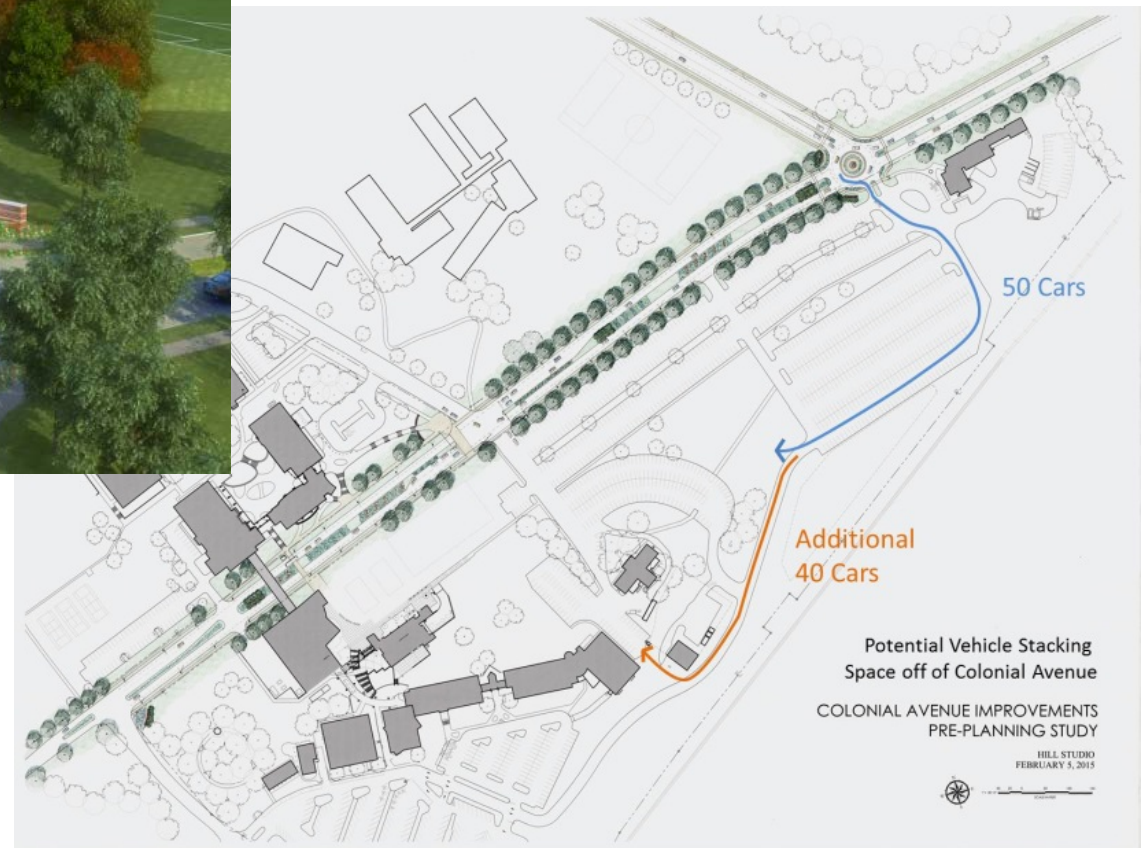
Above, the removal of traffic signal at Colonial and Overland and removal of left turn lanes between Overland and McNeil directs VWCC traffic into the existing campus outer loop drive. Right, diagram shows quantities of cars that can back up flowing into potential future garage entrances, without impeding Colonial Avenue
