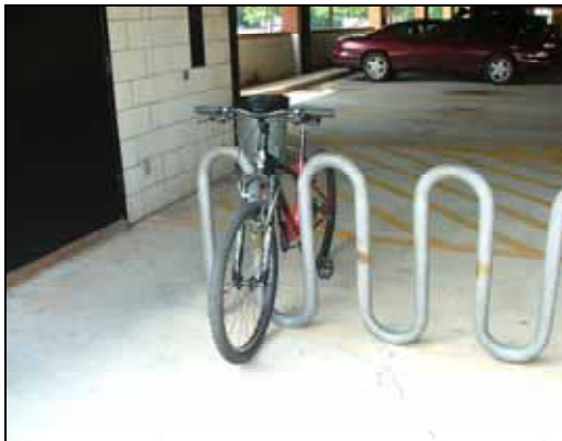
Figure 5.16: Wave design bike rack.
