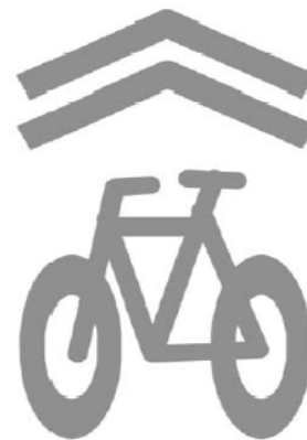
Figure 5.12: Bike-and-chevron or “sharrow” shared lane pavement marking.
