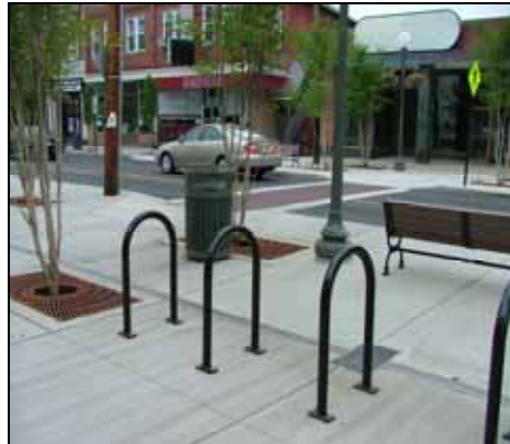
Figure 5.17. Inverted –U design is the preferred style of bicycle rack.
