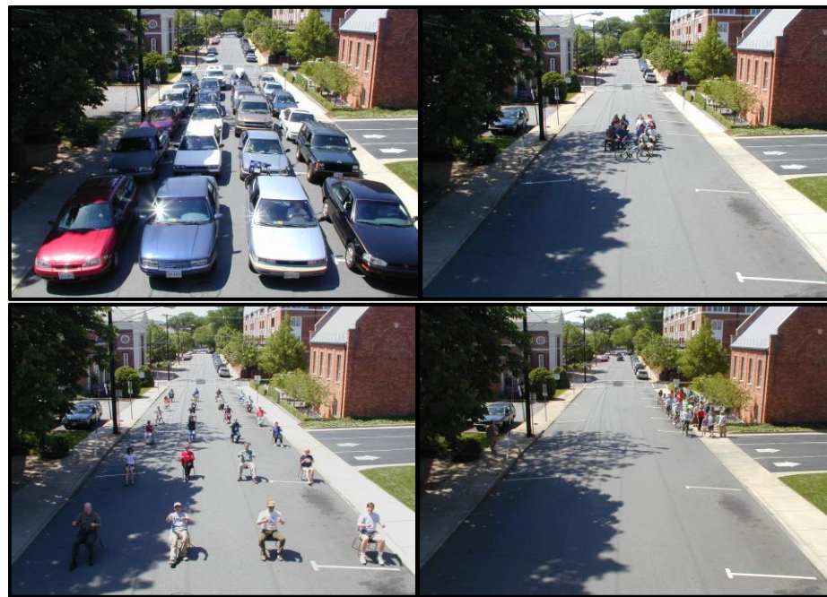
A congested road with single-occupant vehicles (top left) may not serve very many people given the space required (bottom left). The same number of people require less space when able to travel by other modes: transit (top right) and walking/bicycling (bottom right).
