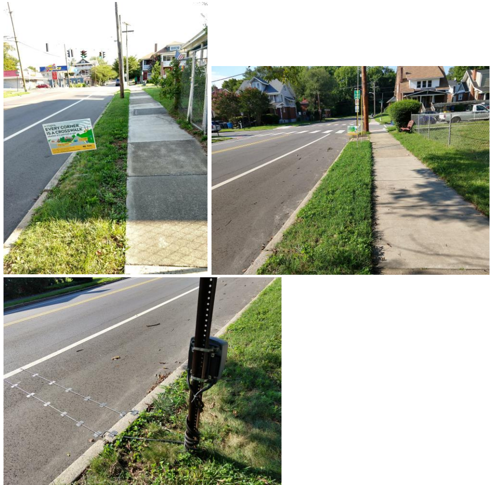
Counter locations on the east (top left) and west (top right) sides of Main Street, and the counter and tubes installed (bottom).
