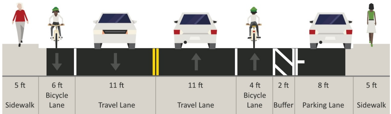
Proposed bike lanes on Ridgeway St from Fifth St to Roxbury St with one sided parking
