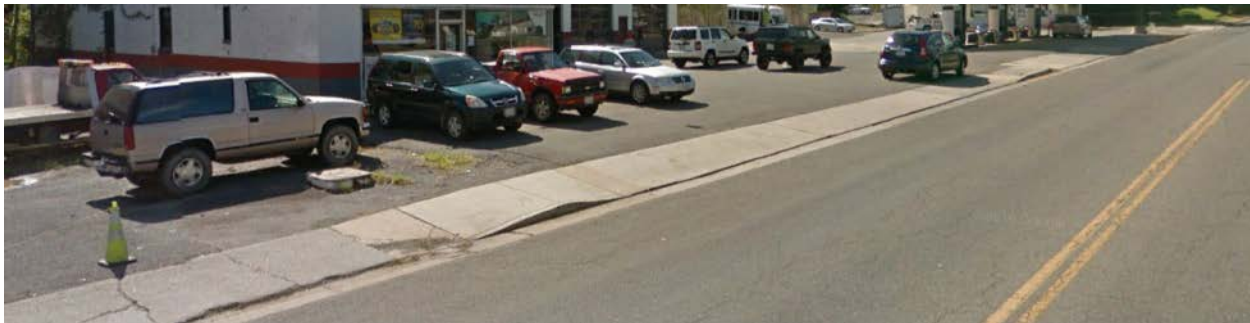
Example of wide and closely spaced commercial entrances on W Ridgeway St
