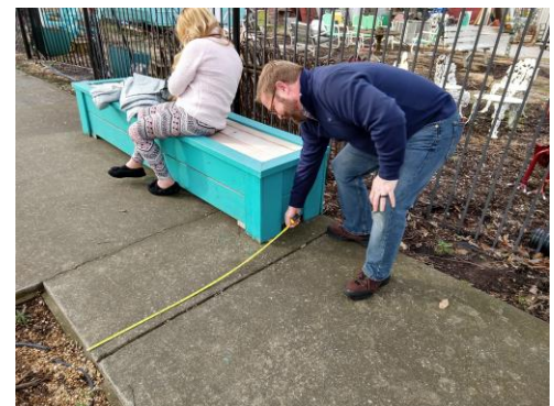
Figure 3. As the Downtown Plan is implemented, care should be taken to protect the 4-foot walkway from encroachment by street furniture
