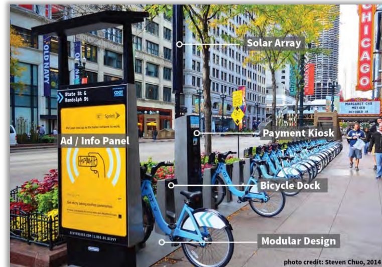
Figure A.2-2 | Typical Dock Based Stations
