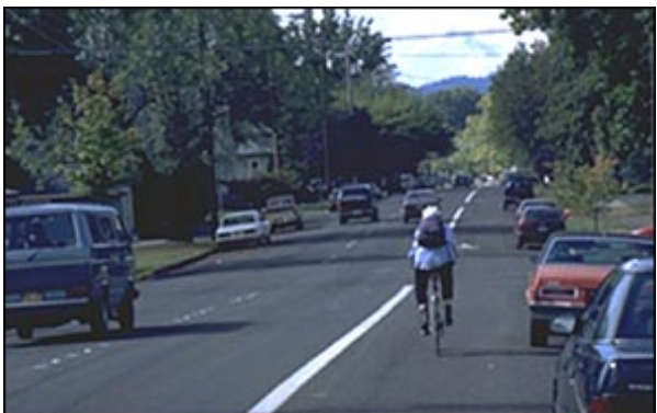
Figure 15. Operational Example 3 - one-way multilane street with a shared bicycle/parking lane in a residential area.
