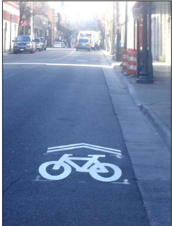
Sharrow (shared lane marking) on Church Street in downtown Roanoke. Markings also serve as wayfinding for on-street bicycle connection between Mill Mountain Greenway and Lick Run Greenway
