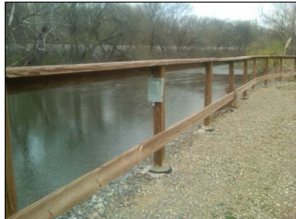
TRAFx infrared trail counter and housing
