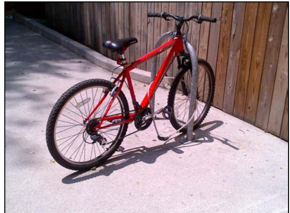
Improper use of inverted-U type bicycle rack in downtown Roanoke
