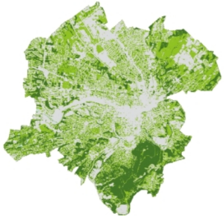
A classified high-resolution satellite image of Roanoke, VA shows the landcover features needed to calculate the air quality and stormwater benefits of trees. Dark green represents tree cover, light green represent grass and open space, and gray designates impervious surface.
